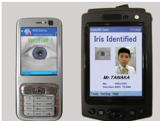
Fig. 8. Iris recognition technology for mobile terminals (OKI introduces Japan's first iris recognition for camera-equipped mobile phones and PDAs, In: OKI Press Releases , 27.11.2006, Available from http://www.oki.com/en/press/2006/z06114e.html )
