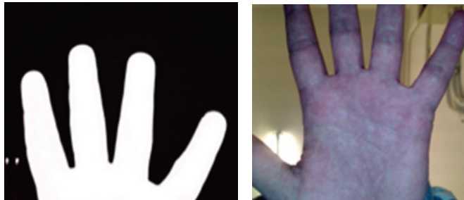
Fig. 4. Left: image acquired by the IR webcam, right: visible image of the hand palm.
